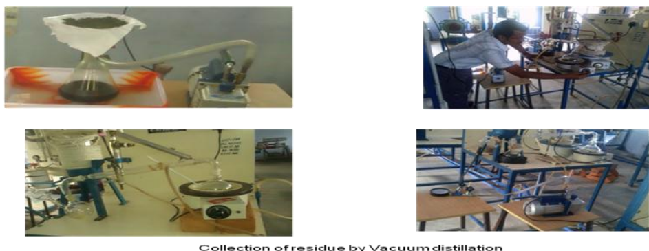
Figure 3: Photocopy Of Evaporation And Filtration Using Vaccum Distillation
